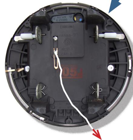
Connect the other end of flexible wire to meter ground if the line neutral is connected to meter ground. If not, connect wire to some other neutral point, such as neutral bar or neutral on a receptacle inside of power outlet box. If installing a USG meter kit, there WILL NOT be a neutral connection to the meter socket ground screw.
